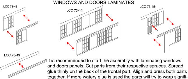
cantly. It is recommended to press the laminated parts in between two heavy and flat surfaces (like heavy hardback books, care should be taken not to allow the laminated parts stick to the books by removing the squezeout [excess glue] and or lining the press with non stick material). When glue has dried the parts will stay flat. Ensure the parts are lined up correctly!
